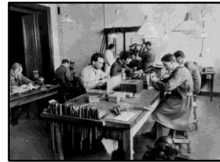
Union Mineral du Haut Katanga (Belgian Congo). Preparing radium tubes from extracted radium minerals.
