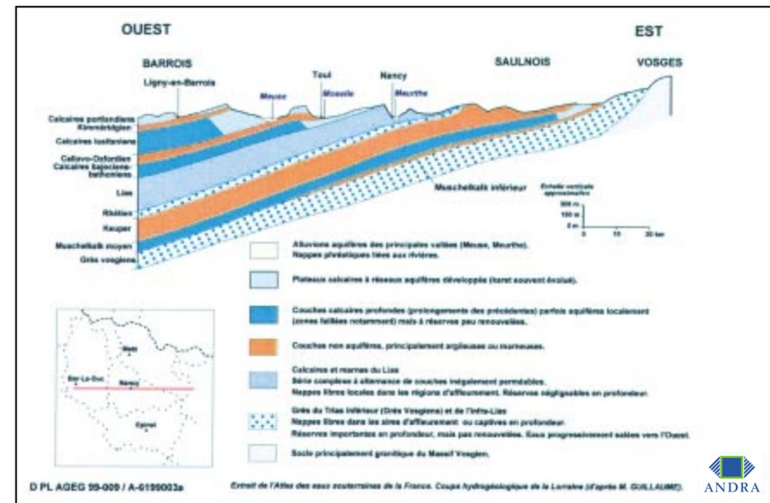
Figure 2-2: Schematic hydrogeological section of the eastern Paris basin
