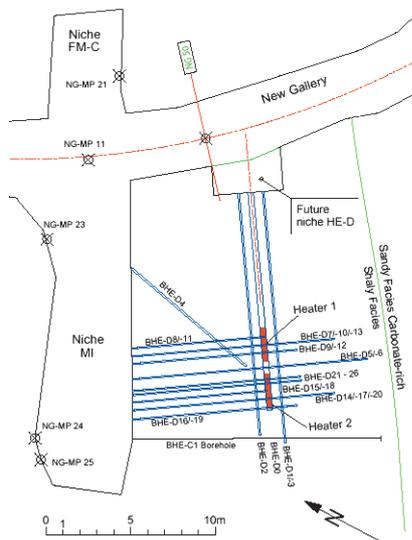
**Figure 1:** Up view of HE-D experiment
