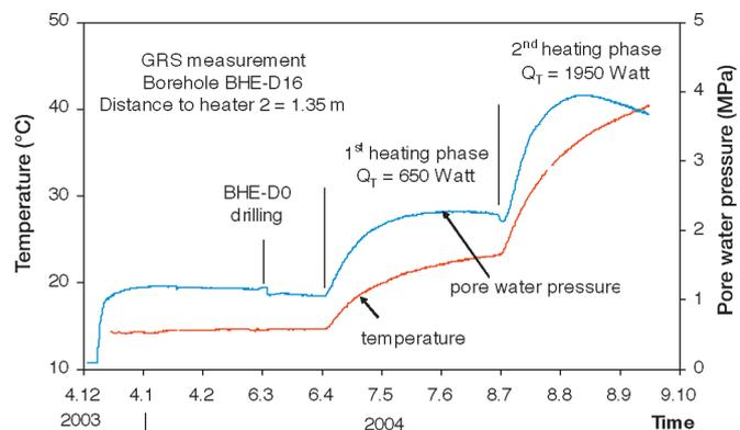
**Figure 2:** Measurements of temperature and pore water pressure during the heating experiment in the Opalinus clay at Mont Terri
