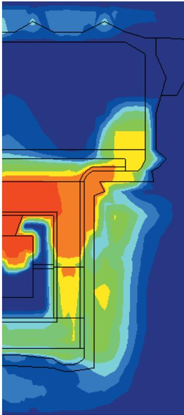
**Figure 1:** Distribution of gas pressure during gas injection test RGI3.
