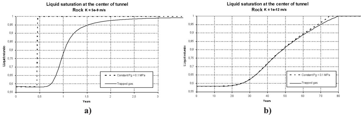
**Figure 2:** Impact on the saturation time of trapped air with different assumptions of rock permeability.
