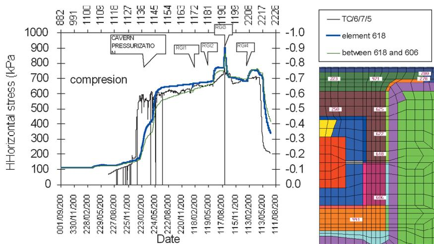
**Figure 2:** Calculated and measured horizontal stresses in layer 6, i.e. in the backfill between the concrete silo and the host rock.
