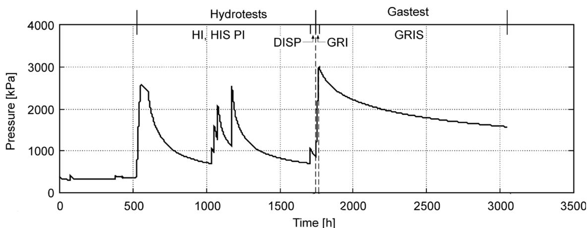
**Figure 1:** Sequence of hydraulic tests and gas threshold pressure tests in borehole BGP4 of the Mont Terri Rock Laboratory
