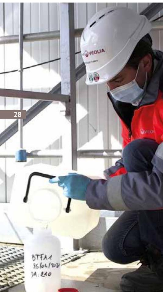
PRÉLÈVEMENT D'EAU DU BASSIN D'ORAGE POUR ANALYSES
